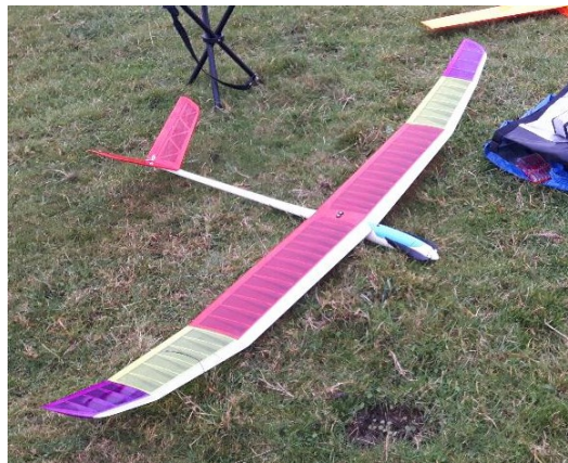
3 - Channel electric thermal glider with 2m polyhedral wing. Ideal for beginners
