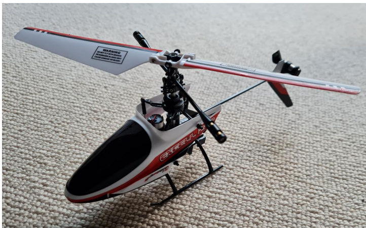
Typical fixed-pitch helicopter
