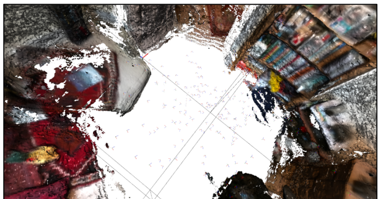
Keyframes seeded throughout the space (the little coordinate axes around the gridlines in the middle of the room show their locations and poses)
