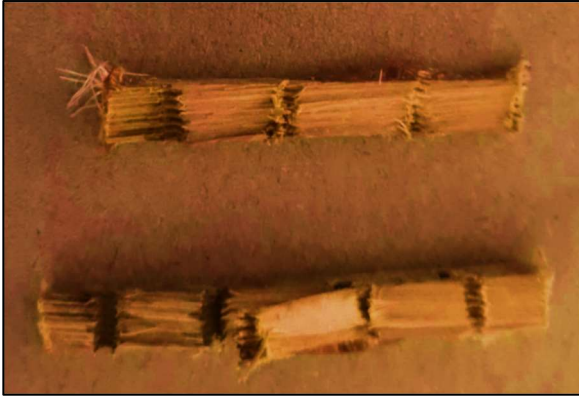
Split Rear Servo Bearer (left) and the Failed Bond on the Front Servo Bearer (right)
