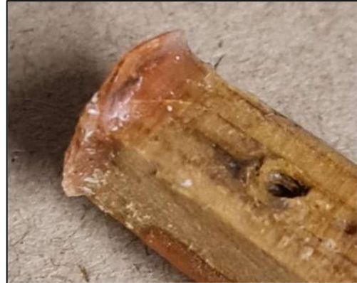
Split Rear Servo Bearer (left) and the Failed Bond on the Front Servo Bearer (right)
