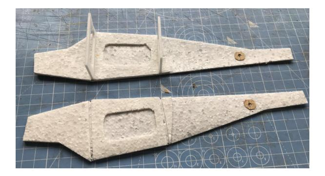
In the picture above you can see the reinforcing discs at the rear motor peg positions. Yes, I should have added these earlier, but forgot!
