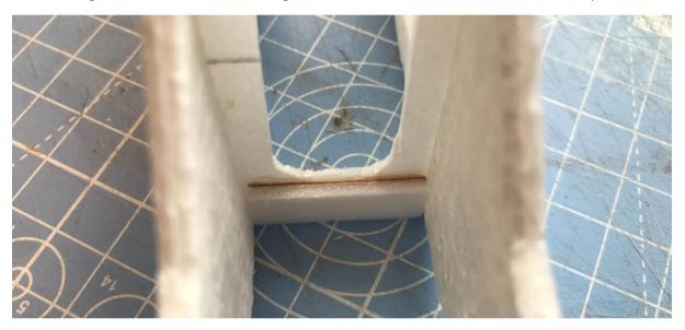
Now it's time to add to top and bottom sheeting, but these are going to include doublers. I started by cutting a piece of foam that would fit between the fuselage sides for the forward underside section. Again, make a card template and check the fit before cutting from foam. This is the doubler that is going to fit inside the fuselage, its glued to a second larger piece of foam that forms the outer sheeting, this second piece is cut oversized for now and will be trimmed to size later.
