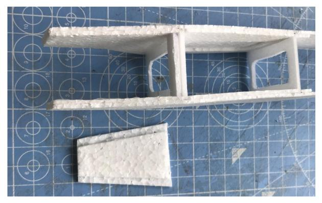
I then glued the composite piece above into place so that it forms both a doubler inside and an outer skin. The outer skin was trimmed to size after gluing. I used PUR for this.
