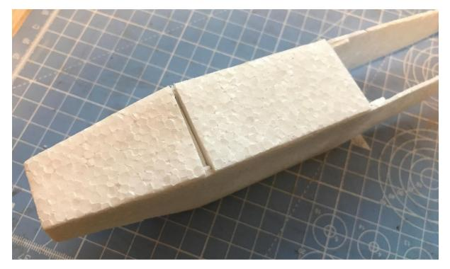
All that remains to be done now is to sheet the upper and lower rear end sections of the fuselage. These don't need the internal doubler, just the outside sheeting. If this were a balsa fuselage I would start by pulling the back ends together and joining these but if you do this with the foam it's all so flexible that it would get bent out of shape when you add the top and bottom, so don't join the back ends just yet.
