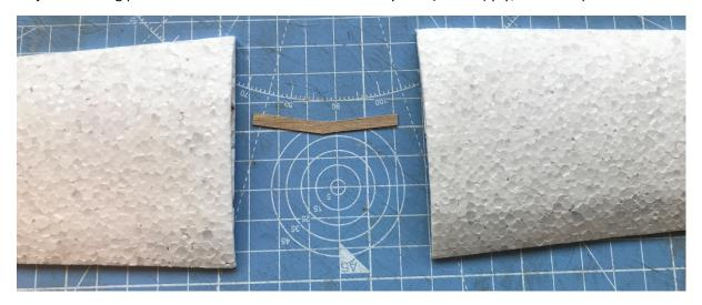
I glued the brace into one panel first, then added the second one later:-
