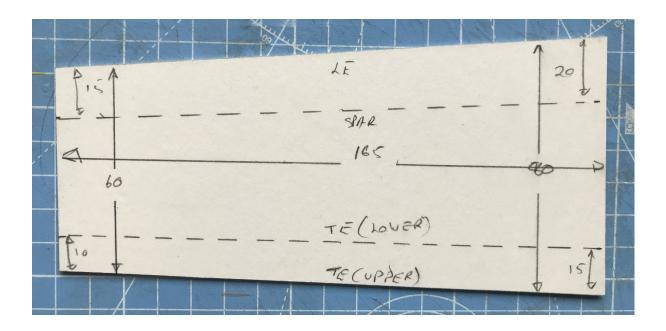
One point to note is that after I took this picture I realised that by making the spar 25mm back from the LE at the root (rather than 200mm as shown) then the spar would be straight through when the panels were joined.
