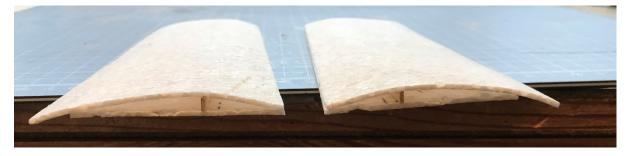
Clearly now the upper and lower wing panels are going to be different, the lower one being narrower. I made the half span 165mm, the root cord 80mm and the tip cord 60mm. The template, with the spar position and bottom panel TE positions marked on it looks this:-
