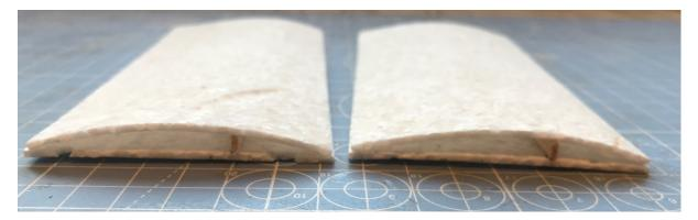
The next step is to put a small radius onto the leading and trailing edges. I used some 600 grit wet&dry, used wet for this.
