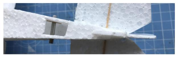
Time to move on to the undercarriage (U/C), but first I fitted a small tailskid which I cut from 2mm Depron, but could have used 1.5mm balsa. There isn't much to the tailskid but it will reduce the drag if you try a 'rise of ground' (ROG).
