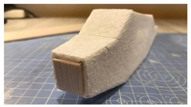
I then glued this (cross grained again) to a piece of 3mm that had been cut a little over the size of the outside dimensions of the nose. I could have stopped there but added a second cross grained piece to make this nose block 6mm thick. The centre of the nose plug was already marked so I then drilled a 3mm hole through the whole lot, for the prop bearing.
