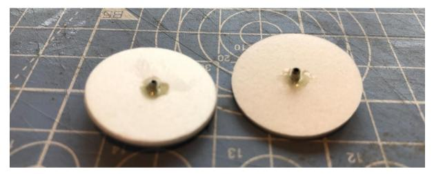
To retain the wheels I used a short length of insulation stripped from some electrical wire that happened to be a tight fit over the U/C wire:-
