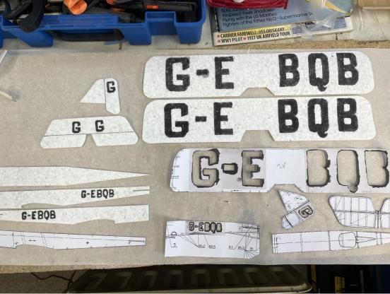
For very small letters such as those on the fuselage sides I found the best method is just cut the stencil to the outer external shape and then use the fine tip to follow the outer shape, paying closer attention to the inside line the pen is making allowing the stencil to
