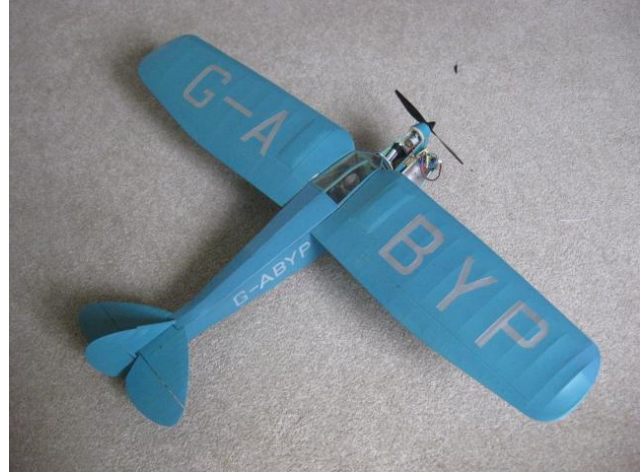
The West Wings Puss Moth converted to small electric power [photo B Dennis]
