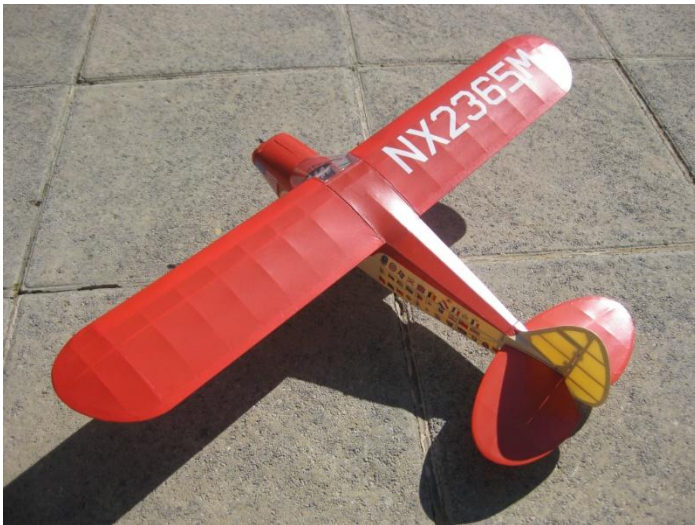
The KK Piper Super Cruiser is a light, slow flyer for a small diesel [photo B Dennis]
