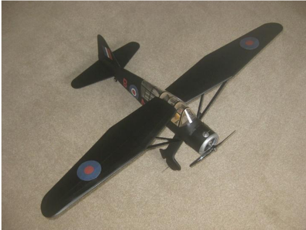
This is a KK Lysander blown up 200% (36") for a small diesel. Don't go bigger or you will need more ribs and formers. [photo B Dennis]
