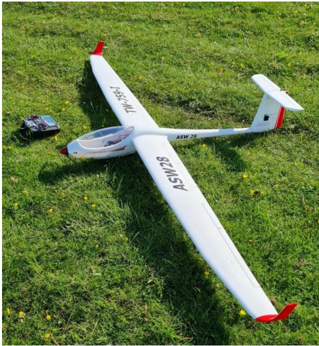
Semi-scale Foamie E-Glider (ASK28). Note the flaps on the trailing edge inboard section of the wings.
