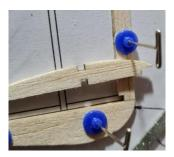
I like to sand the wing trailing edge top surface down slightly to follow the line of the ribs, sticking tape over the ribs to prevent them from being inadvertently sanded. Again, this is unnecessary, but I think it improves the look of the finished wing.
