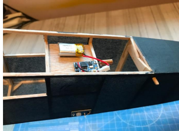
The BMK RTD system is mounted internally under the wing
