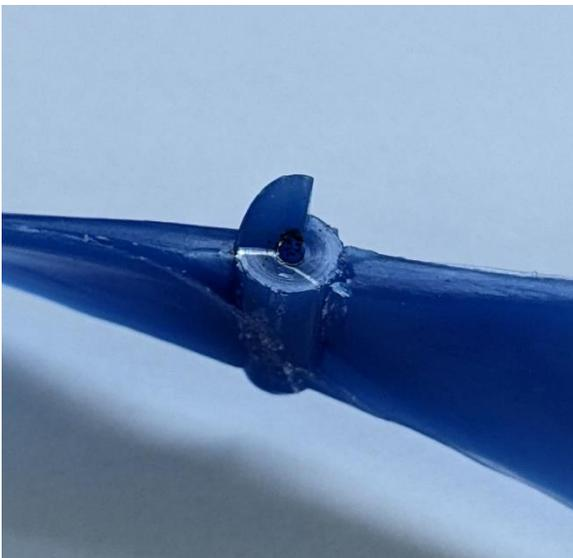
*A standard commercial ramp-type freewheel - the flat edge of the ramp is aligned with the middle of the prop shaft hole rather than the edge, and the hole is square-cut so that a bent piece of wire will not fit properly.*
