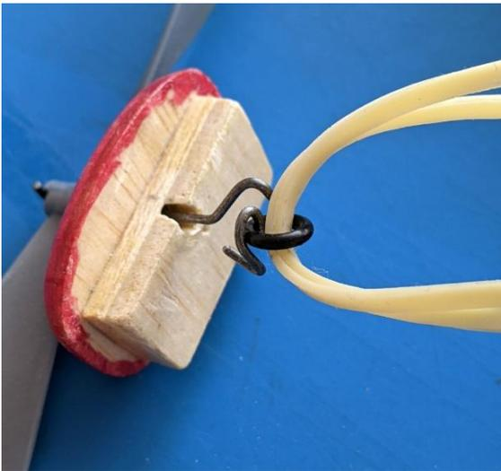
*A reverse-S hook with the rubber captured by an 'O' ring so that the prop assembly can be easily detached for winding. Check The Internet for instructions on how to make one.*
