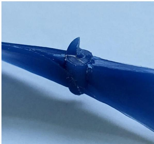
*After a few minutes work with a file and scalpel, the edge of the ramp has been cut back so that the prop-shaft will fit properly, and the edge of the hole has been rounded so that a bent piece of wire will fit.*
