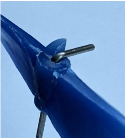
*A modified freewheel ramp with a prop-shaft installed. Note how the prop shaft has been bent to slightly more than 90 degrees so that it fits the sloping ramp.*
