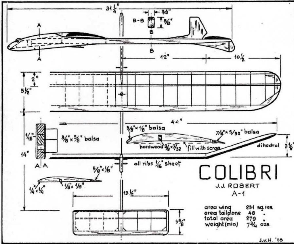
I carry my A1s around in an old trombone case (as you do . . .) which is 32" long, I made the wing of the *Colibri* two-piece. I used a single 10SWG (3mm) wire joiner. I doubled up the spruce spar around the middle and epoxied the tubes to take the joiner to this (Fig 4).
