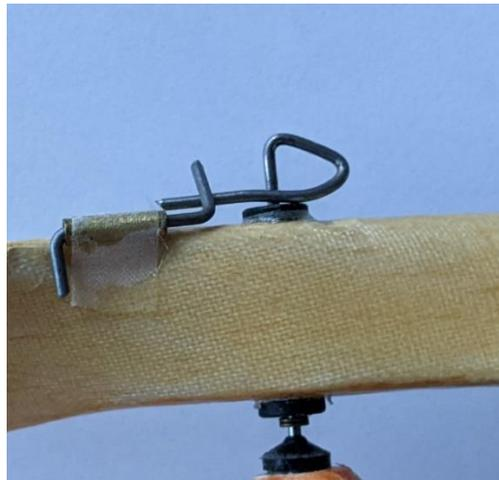
*A Garami clutch shown in the engaged position. The engagement is very positive, but the lever-in-tube part of the mechanism must be manually engaged as the winder is removed.*
