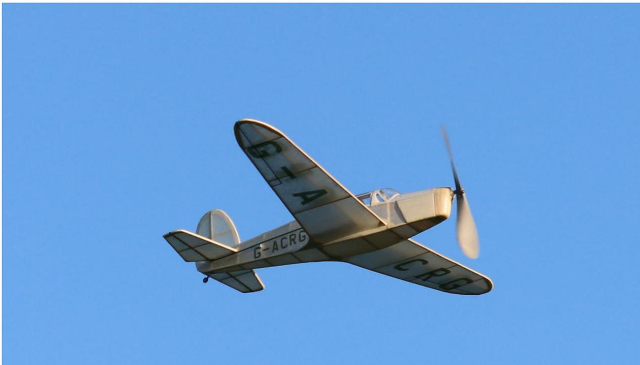
*Author's Pseudo Dime Scale B A Eagle is built from heavy (12 lb cu ft) strip wood and light (6 lb) sheet, weighs about 12 grams empty including nose weight, flies for 60+ seconds on 1200 turns.*
