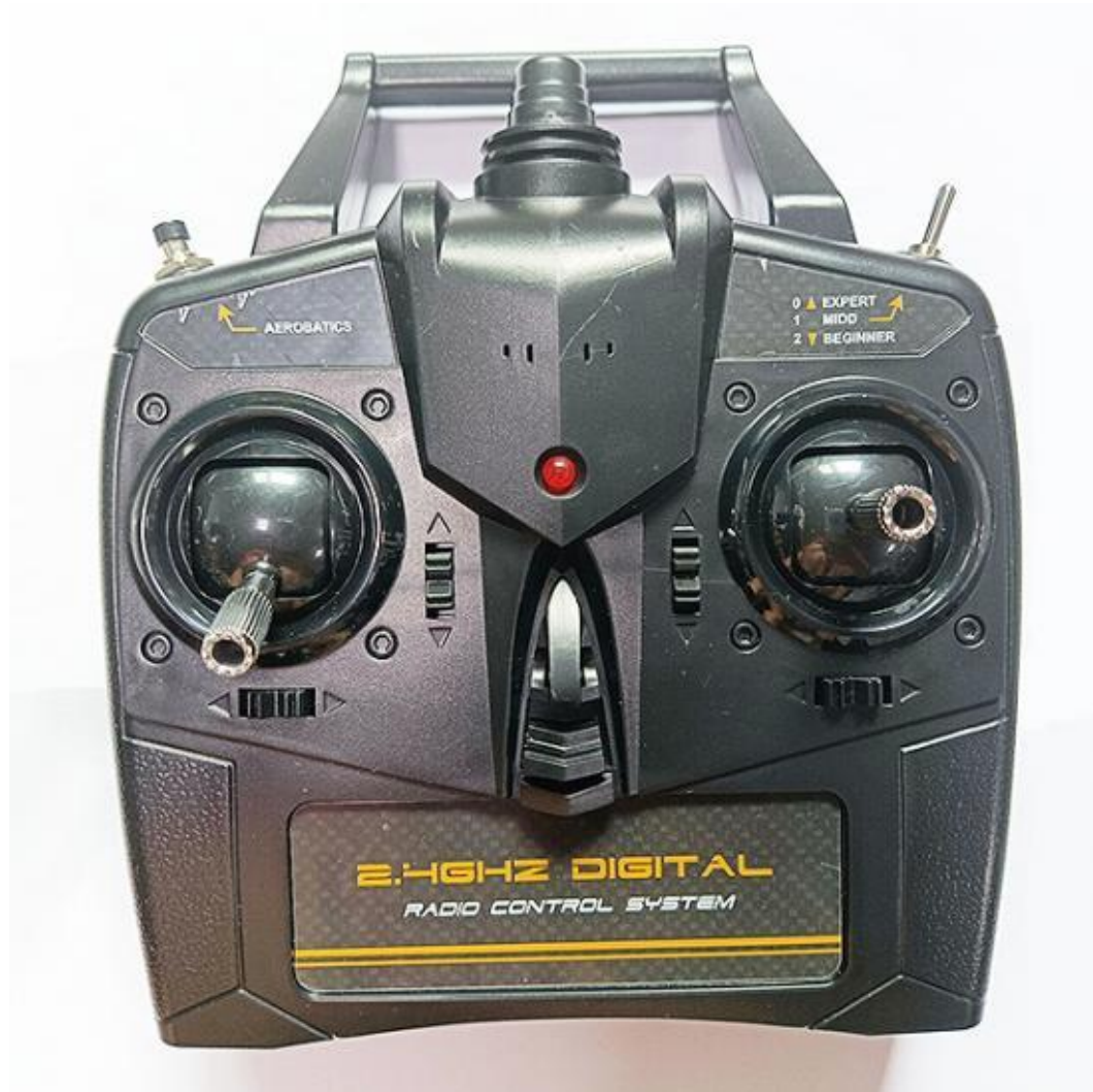
A Typical RTF Transmitter; Note the 3-position 'Expert, Intermediate and Beginner' switch (top right), and the automatic aerobatic manoeuvre button (top left). Note also the lack of adjustable rates, and no computer power for expo.
