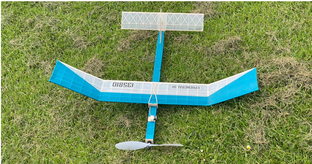
Ephemeral01a. Made up from discarded components from Ephemeral01. It's a bit untidy with several repairs, but my best performing P30 to date!
