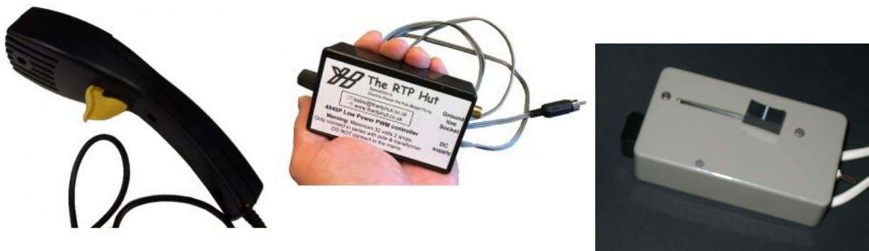
Controllers Left to right - Scalextric type, RTP Hut Pulse Width Modulation (PWM) controller, Oxford Controller
