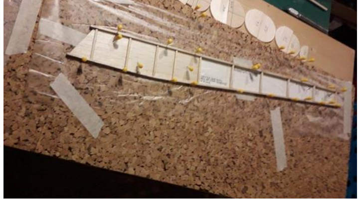
The front of the fuselage sides were made up as per the plan, using 1/16th sheet and glued internal strips. Personally, I would have just built at final thickness. The first fuz side taking shape showing the front side in place plus the longerons and spars.
