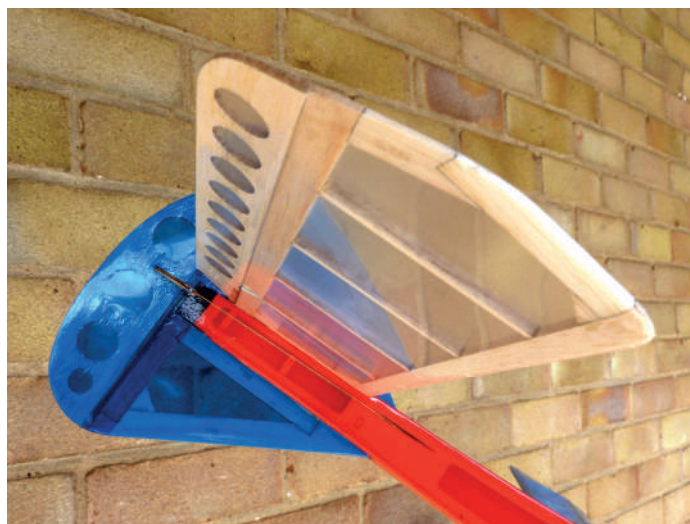
Lulu RC Lite rudder and tailplane details.
