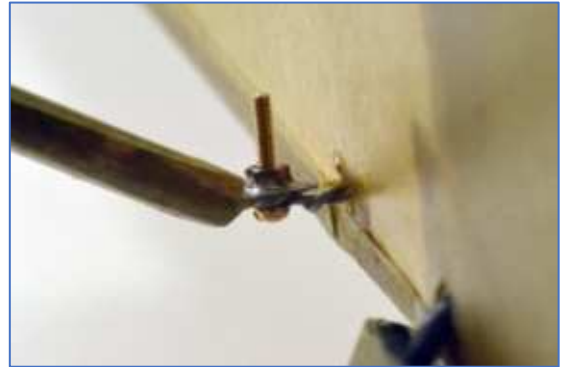
Strut to fuselage fixing. The bolt (12BA) goes through a twisted wire loop into the fuselage and a nut soldered to a tinplate tab at the end of the strut.
