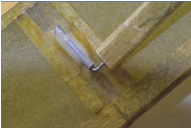
Strut to wing fixing. Wire on the end of the strut into an oversized piece of tubing epoxied to underside of wing.
