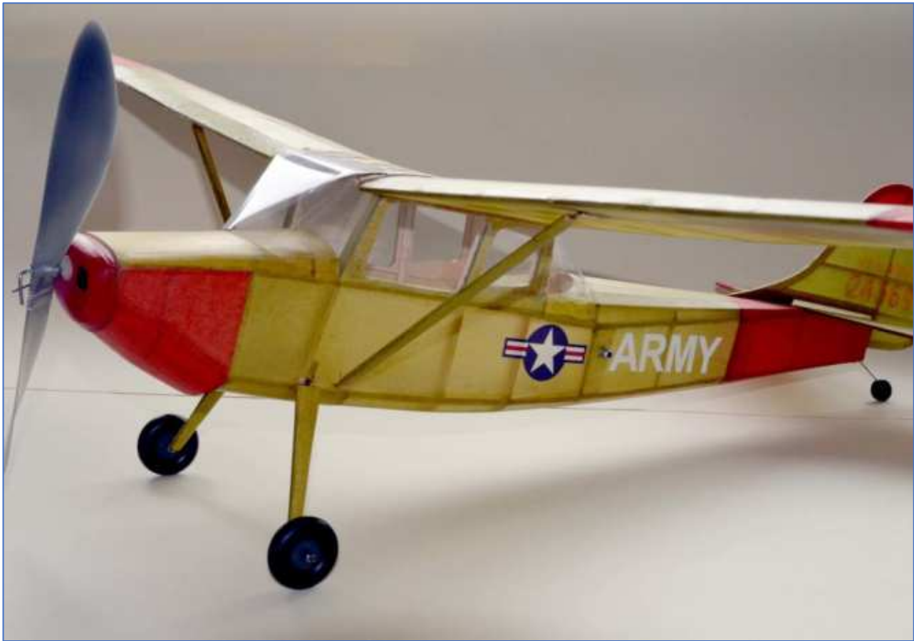
The finished model. Note the forward motor peg position. It was originally further back where the red area starts.
