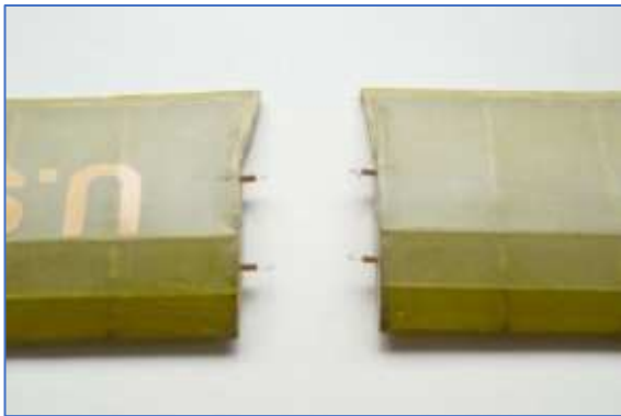
Wing dowels. Keep them short. Wire hooks made from 22 gauge guitar (top E) string.
