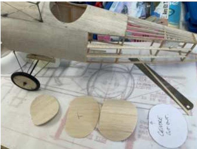
3 layers for the cockpit coaming
