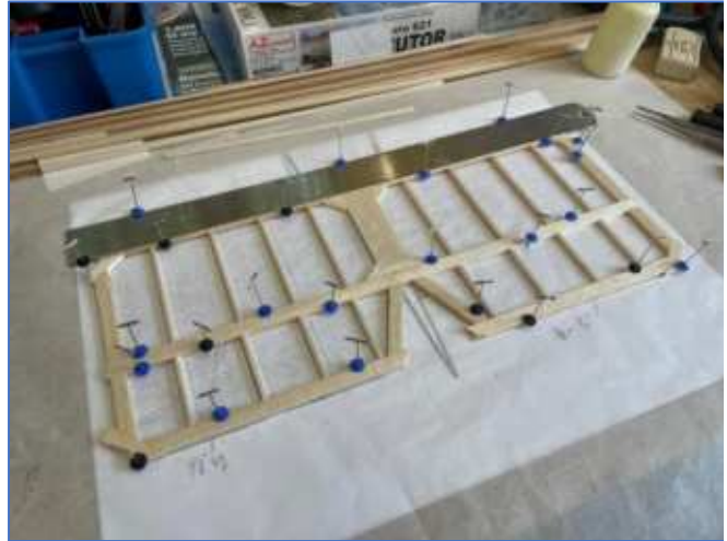
Flat-plate tail with dowel LE
