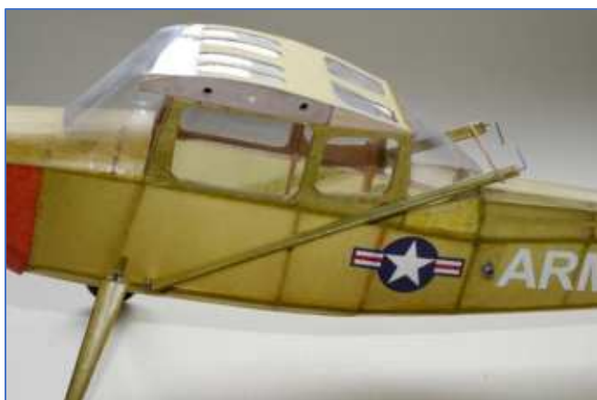
Struts folded back for storage, there is no need to ever unscrew those 12BA bolts, you only need to fiddle with them (and drop them several times) once.
