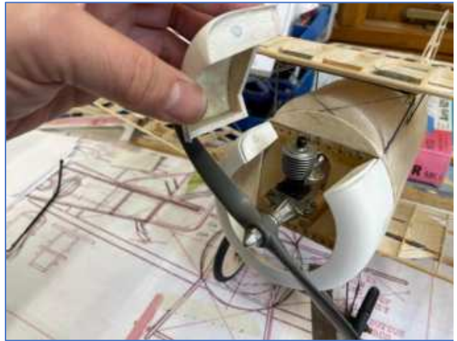
Cowling with removable top section
