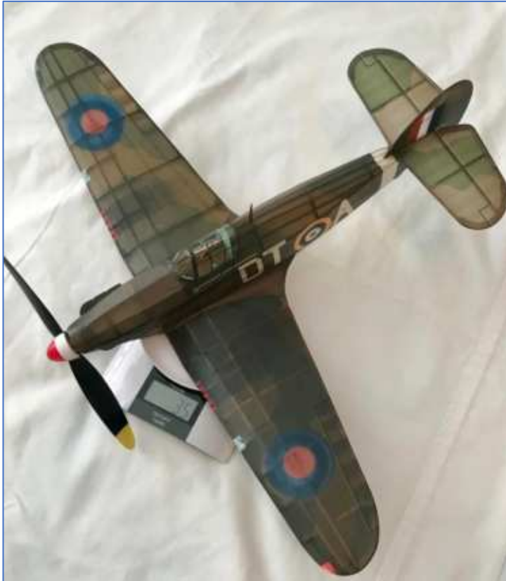
A dime scale 16" Comet Hawker Hurricane enlarged to 24" - note the minimal weight (35 grams) shown on the scales.
