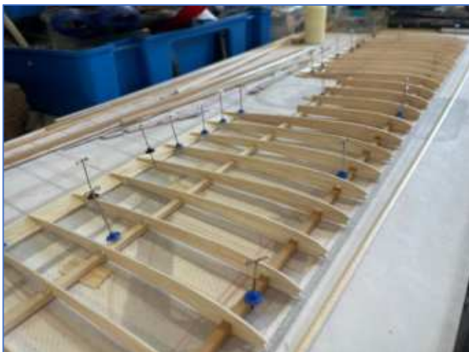
Top wing construction with dowel LE
