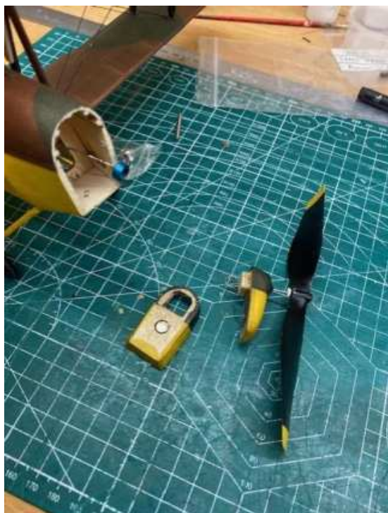
First, saw off the nose with a razor saw (!!)
