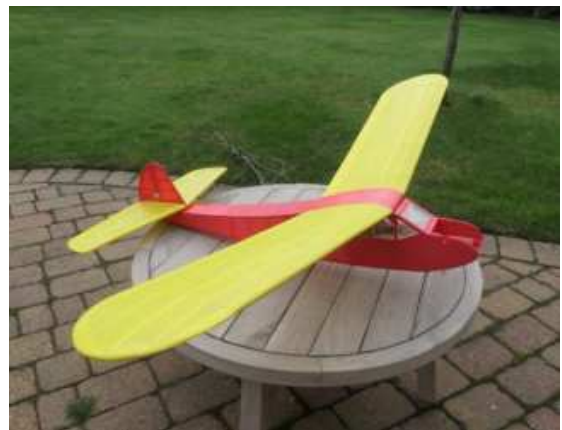
Sunduster - my latest build and first effort with Eze tissue over laminating film
