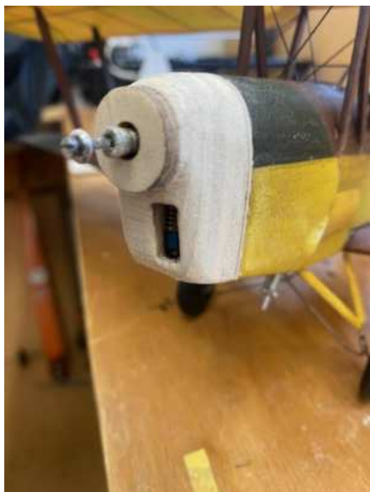
Make a new cowl to fit, held on by magnets.
