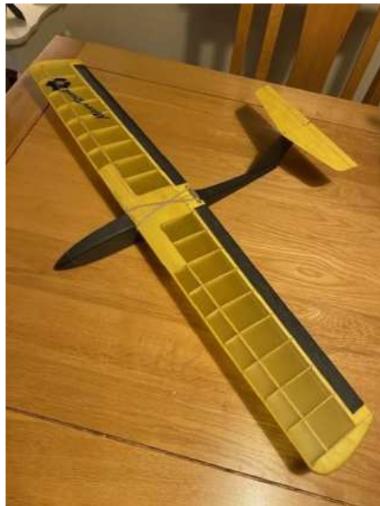
Micro Runt slope soarer from Angelwings, can be bungeed. Flysky 2ch aileron and elevator
