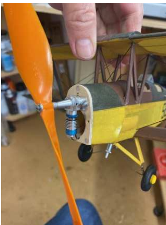
Then install the motor (Gasparin GM 63) on a ply plate, CO2 tank sits behind cowl, filler is between UC legs
