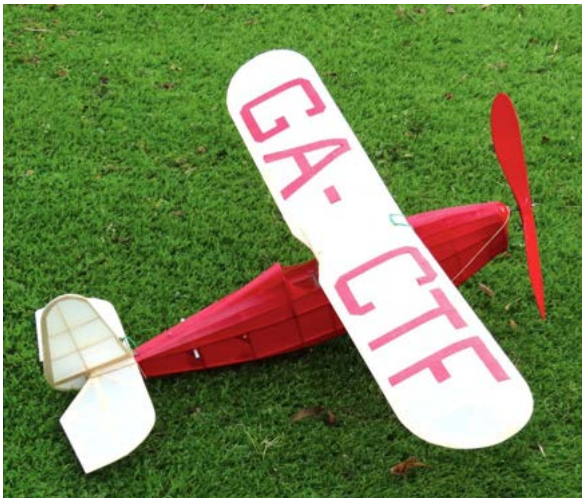
Andrew Longhurst's 30" Comper Swift enlarged from a Veron plan [Andrew Longhurst Photo]
