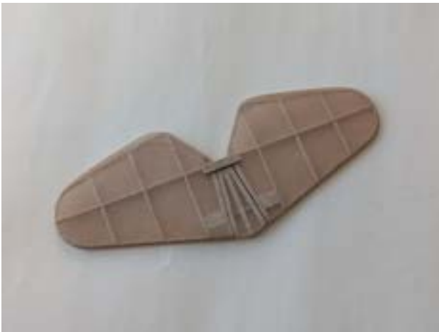
Underside of tailplane converted to D/T operation using a short length of 1/16" tube
