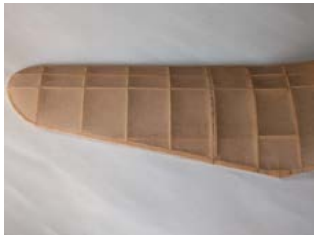
The wing panel in place. In this particular case, a pair of 6mm magnets were used to fix the outer panel in place, and it's a bit too strong. 3mm magnets will be used in future.
