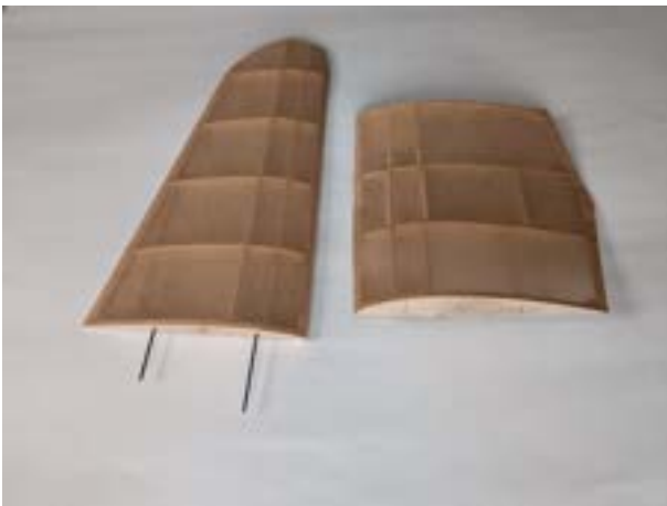
1.6 mm carbon tubes are permanently fixed in the outer wing panel. Note differing lengths to ease fitment
