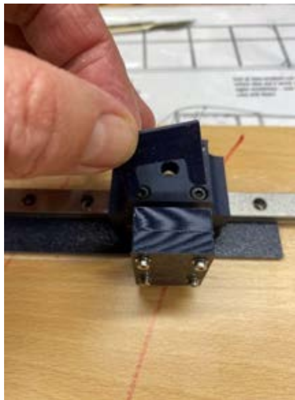
Components screwed together showing where the U-shaped spacer(s) fit
